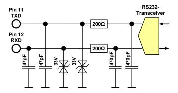
The RS232 port enables a direct, serial connection between the inverter and a PC. You will find the configurations for this in the manual *SW-FW-SHC3\_Firmware\_download.pdf*
