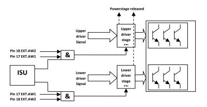
To enable the output stage, pin 3 EN must also be high.
