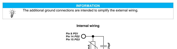
The pins 8, 14 and 15 are each connected with pin 1 GND via a reversible fuse (PTC) and are thereby protected.
