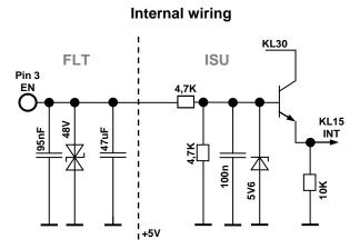
If voltage is applied at pin 2 and pin 3 = high, this effects the start-up of the controller. Communication with the inverter is thereby enabled. If additional HV voltage is applied, this effects the activation of *Ready* mode. The internal device logic is only fed if pin 3 = high. This is also the case if HV+ and HV- are already applied in high voltage. Pin 3 has the function of terminal 15.
