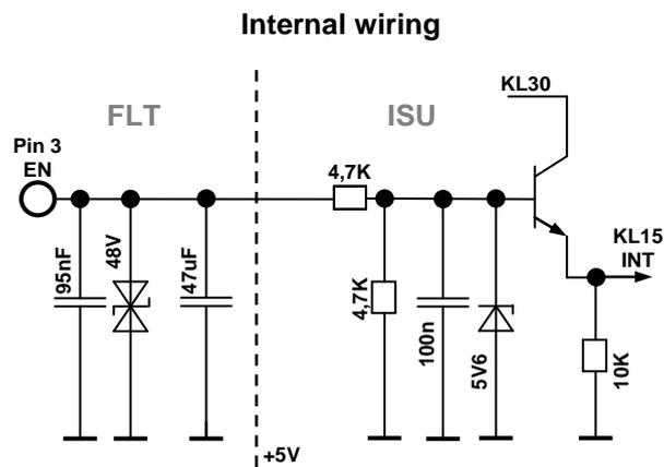
If voltage is applied at pin 2 and pin 3 = *high*, this effects the start-up of the controller. Communication with the inverter is thereby enabled. If additional HV voltage is applied, this effects the activation of *Ready* mode.
