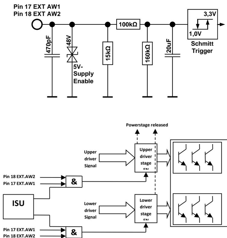
To enable the output stage, pin 3 *EN* must also be *high*.
