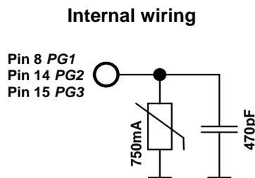
The pins 8, 14 and 15 are each connected with pin 1 *GND* via a reversible fuse (PTC) and are thereby protected.
