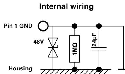
Direct ground connection of the inverter's control electronics.
