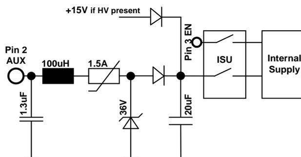
**The internal 5 V supply is generated with this pin and offers the following possibilities:**
